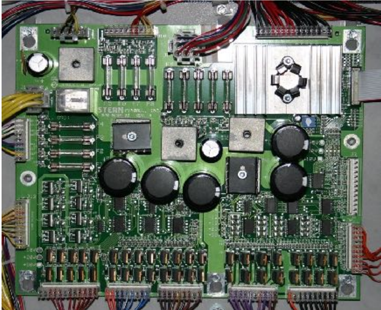
I/O Power Driver PC Board
